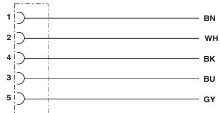
Contact assignment of the M12 socket
